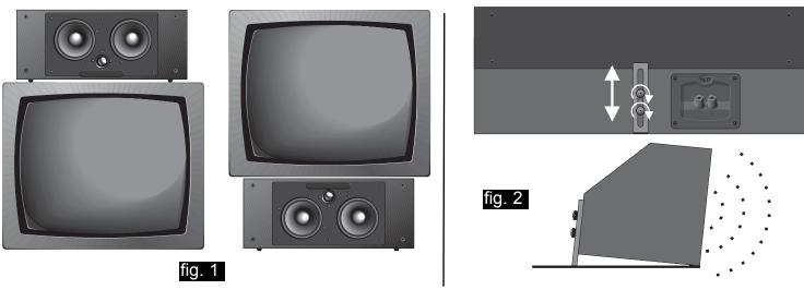
When installing the VS-2a as a center channel speaker, it should be placed directly above or below the television, as close to the screen as possible (fig.1). The speaker should *always* be placed so that the tweeter and absorptive foam strip are facing the screen. The VS-2a is magnetically shielded and will not distort the picture's color.
